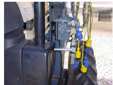
Fully reverse the tractor, fit the covers to the quick release valves and replace the fixing bolts and pins on the proper points of the column of the loader.
