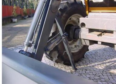
Adjust the height of the shoes such that the bases on the columns are positioned in line with the connection inserted into the tractor.
