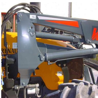
Fully reverse the tractor and fit the covers to the quick release valves.
