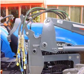
Reverse the tractor slightly until it is possible to fully re-lower the shoes of the accessory to the ground.
