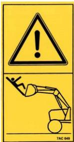
DO NOT GET INTO THE LOADER'S BUCKET, AS THERE IS A DANGER OF FALLING FROM AN ELEVATED POSITION.
