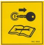
TURN OFF THE ENGINE BEFORE PERFORMING MAINTENANCE.
