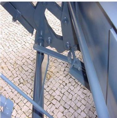
Close the hydraulic cylinders to allow the lower points on the accessory to connect to the matching points on the automatic connector, and to lock the automatic connector's lever.
