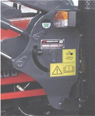
On the H4 model, move the disconnection lever downwards.
