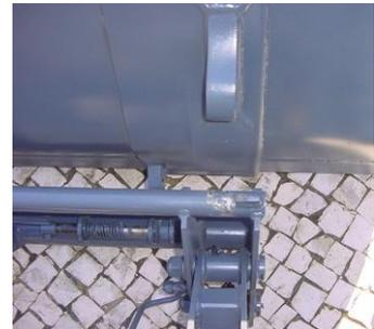
Fit the upper bar of the automatic connection into the upper hooks of the accessory.
