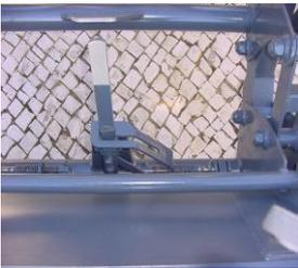
Move the automatic connection lever to open the connection points.
