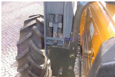
Check that the fixing bolt is correctly placed in the disconnection position.
