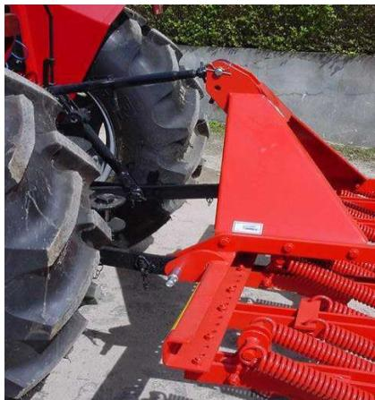
Place the 1st and 2nd points of the tractor's connection arms over the equipment's trunnions and fix the bolts properly in place. Connect the tow bar to the 3rd point and adjust so that the front and rear tips are the same height above the ground.
