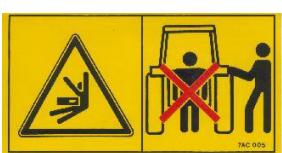
KEEP CLEAR OF THE MACHINE. DANGER OF CRUSHING.
