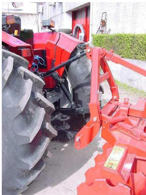
Place the 1st and 2nd points of the tractor's connection arms over the harrow's trunnions and fix the bolts properly in place.
