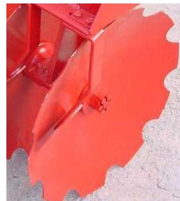
The scrapers must be adjusted such that they are as close as possible to the discs without affecting their free movement.
