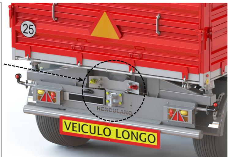
"When coupling the 2nd trailer, ensure that all hydraulic and/or pneumatic connections are properly connected, and that the systems operate correctly. Always test the systems before moving off. Ensure that the eye's coupling bolt is installed correctly, and with the safety pin fitted."
