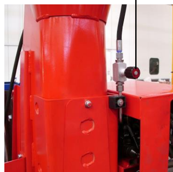
Regulator positioning in the machine with vertical extension of 0.20 m
