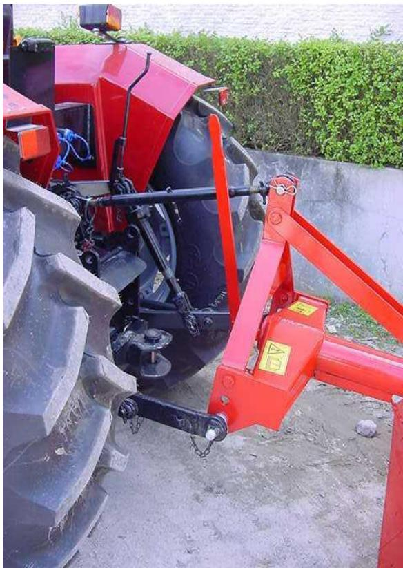
Place the 1st and 2nd points of the tractor's connection arms over the rear mounted grader's trunnions and fix the bolts properly in place. Connect the tow bar to the 3rd point and adjust so that the equipment is longitudinally level.
