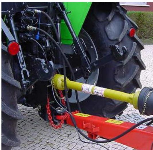
First check that the tank is in good operating and safety conditions, then engage the draw bar with the tractor and fix the bolt in place with a pin.
