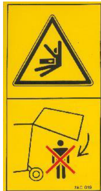
DANGER OF CRUSHING. TIPPING BACK DOOR.
