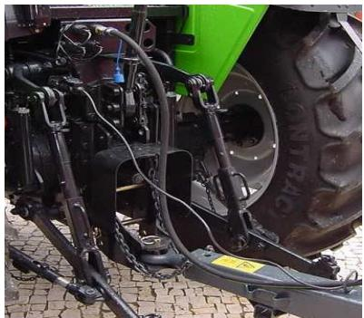
First check that the tank is in good operating and safety conditions, then engage the draw bar with the tractor and fix the bolt in place with a pin.
