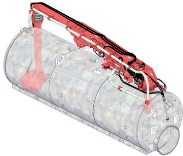
DORSAL ARM WITH 3 ARTICULATIONS, PURGE KIT AND PRIMARY SIPHON
