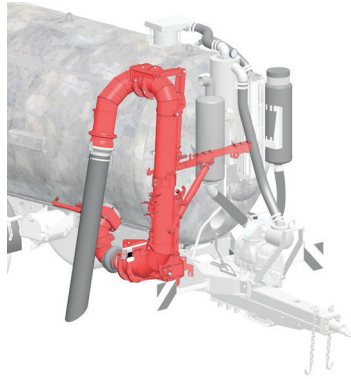
HYDRAULIC ARM WITH 2 ARTICULATIONS, SIZES M, L AND XL
